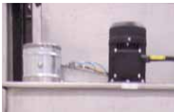
Blow-off fan with integrated heating
